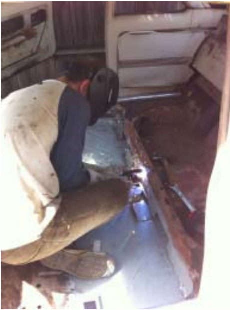
Here is DJ welding in replacement floor panels.
