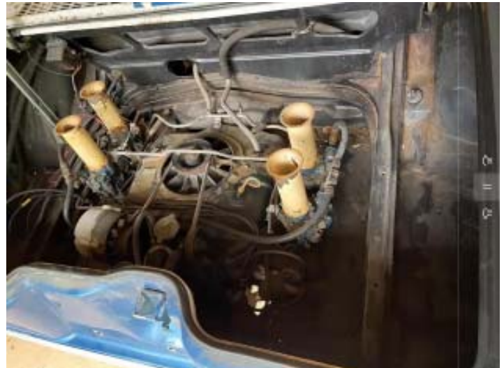
Special blue painted carbs with velocity stacks.
