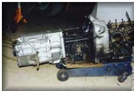
It's a bit longer requiring some modifications to the rear seat area. He ran the linkage below the trans so the floor remains flat. It's a nice combination
