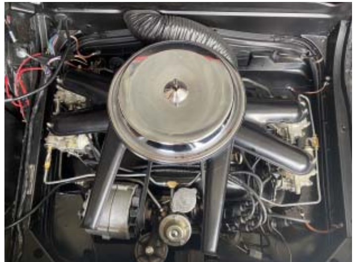
Bruce has replaced the 110 with a period correct 140 he already had. You can see the new wiring harness from Clark's.
