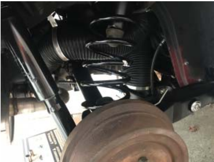
The suspension was gone through, cleaned up and painted. Rubber parts were probably replaced with Clark's stuff.
