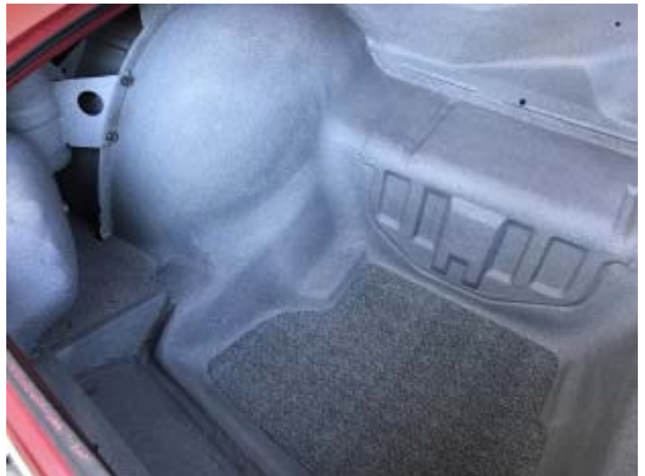
The trunk area has been cleaned and repainted with splatter paint.
