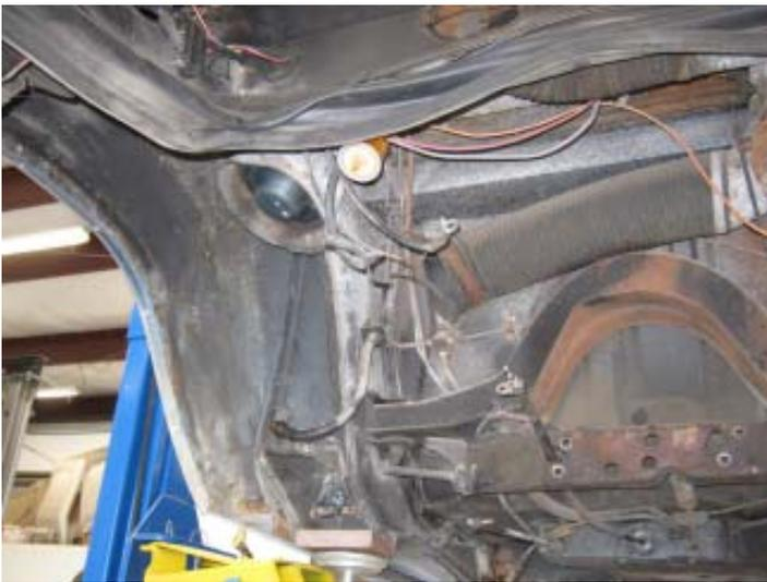
Here we have removed all of the suspension components. Looks pretty bare doesn't it? Now you can easily get the the heater ducks and blower motor!
