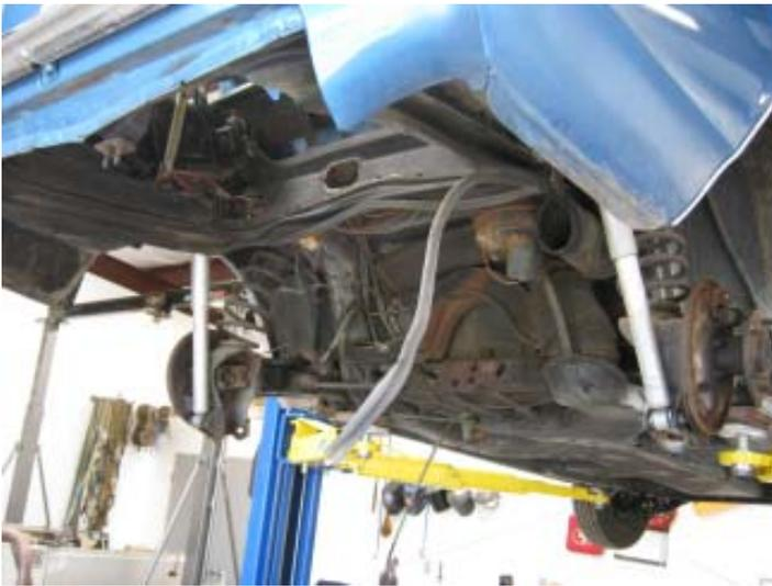
With the engine removed, see how accessible the suspension components are? The weather strip [ping hanging down will be replaced.
