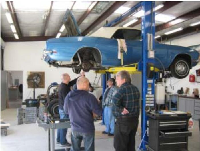
Here we are looking over the job at hand. Notice how Don has added a strap to tie the car frame to the lift. Just in case that without the engine the car may tend to tilt forward. Safety first!
