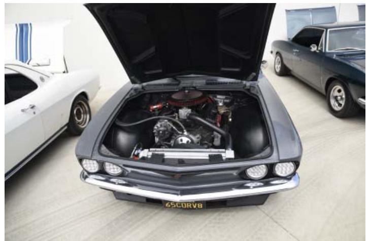
Bill Schaffer's Corvair with a front mounted Corvette LS V-8!
