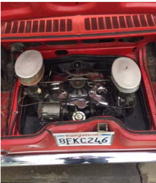
A very clean 140 installation. It looks like an electric fuel pump is installed on the left-rear carb (or maybe that's a fuel filter?).
