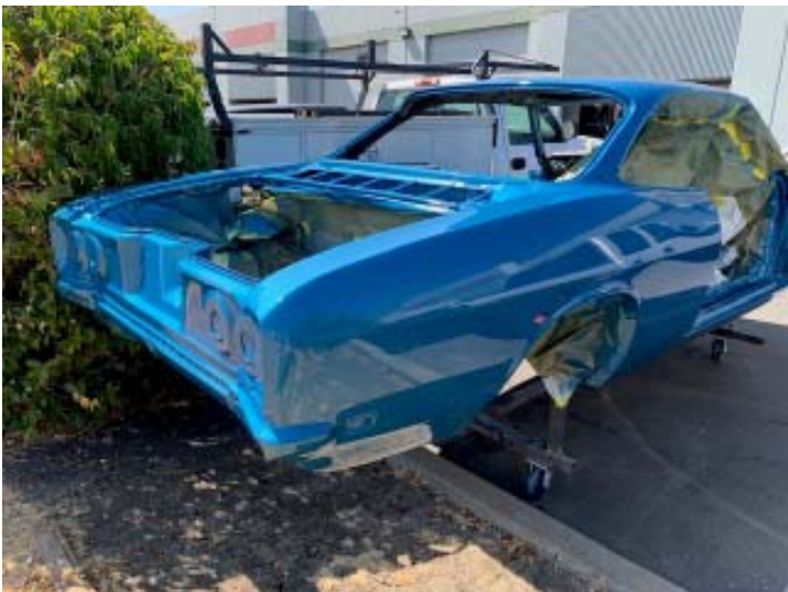
Here the masking paper is being removed.
