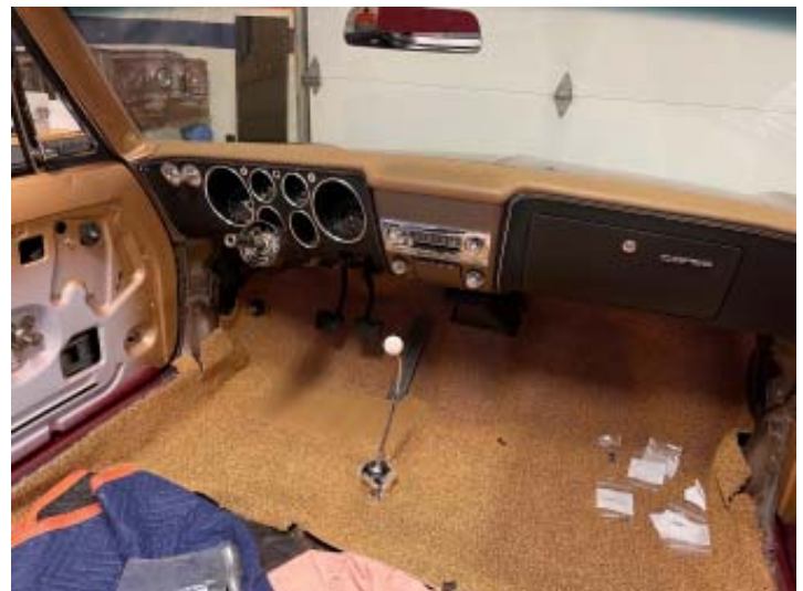
Bruce is now starting to work on the interior. Floors were already in great shape. Here the dash, glove box, and carpets have been installed. Bruce was able to find a NOS Corsa dash.
