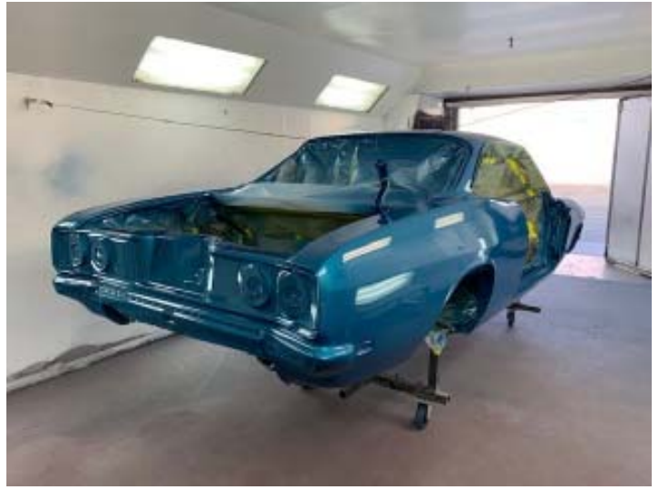
Here the body is being painted. The plan was to use 2 coats of Blue and then 5 coats of Clear.
