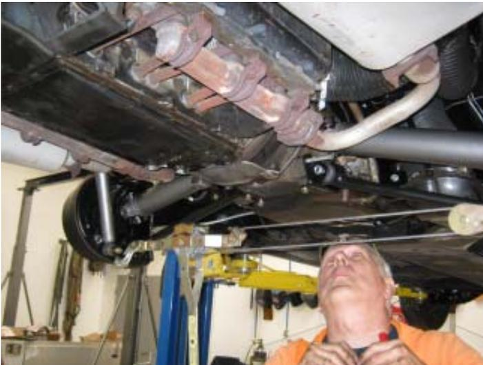
Here you can see the come along that Don used to pull the wheels in just a bit. Don is checking the alignment of the brackets that hold the bottom control arms to the trans.
