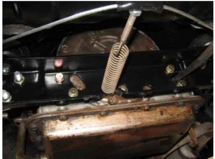
You can clearly see the four bolts that secure the front on the motor to the cross member. The bolt holes are just slightly oversized so some jockeying is required to get the holes lined up so the bolts can be started..
