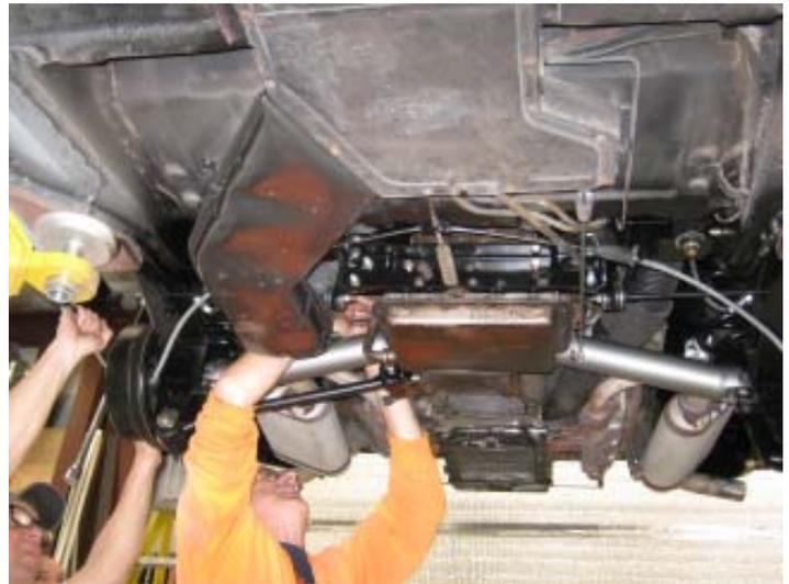
Here we see Don tightening the bolts that hold the U-joints. Lane is using a crowbar to prevent the axle from turning. It is certainly easier if you have help!
