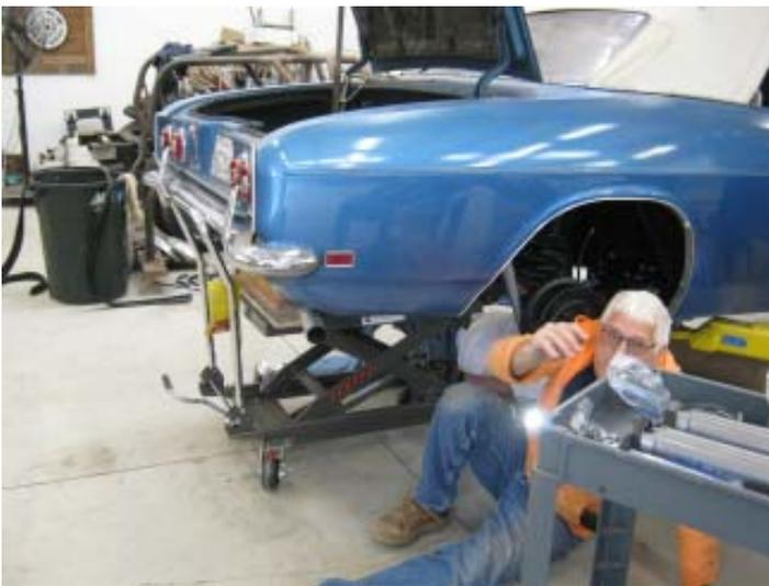
The engine has finally been positioned. It took a bit of jockeying to get the engine to fit between the front and rear mounts. The next step will be to get the holes lined up.
