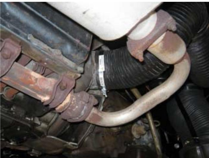
Now that the engine secured, we can turn our attention to the heater hoses. The internal spiral spring wire makes these difficult to connect. Don had some dry Teflon spray lub that he used and this made it easier to connect up the hoses. Once they were connected the hose clamps make sure they won't come apart.
