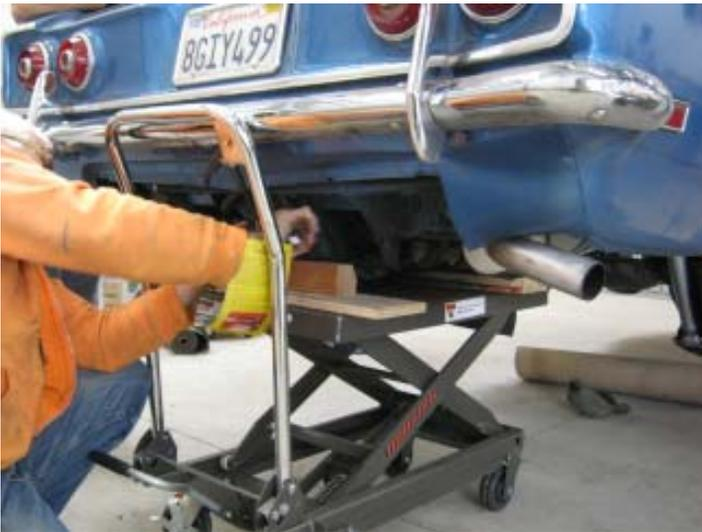
Here Don is tightening the nuts on the rear motor mount.
